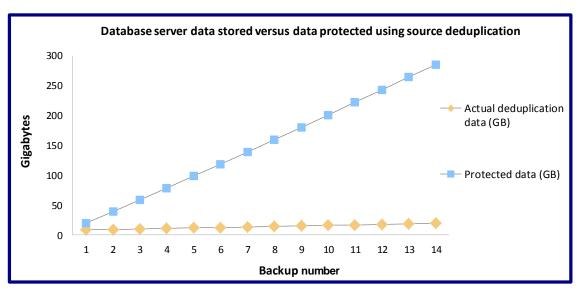
Figure 2: Comparison of protected data versus the actual data stored from our 2-week database backup simulation of a SQL Server database.
