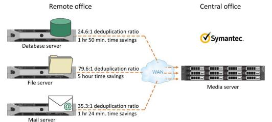
Figure 1: Symantec Backup Exec 2010 R3 significantly reduced the amount of data storage and time needed for data backups in physical environments.
