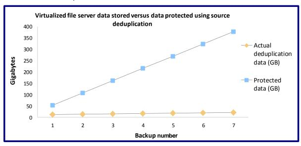
Figure 7: Comparison of protected file server data versus the actual data stored from our 7-day virtualized file server backup simulation.
