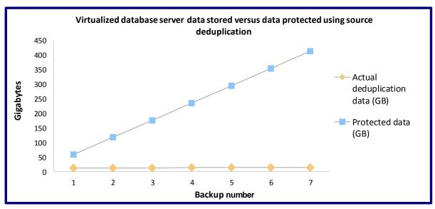
Figure 6: Comparison of protected data versus the actual data stored from our 7-day database backup simulation of a virtualized SQL Server database.
