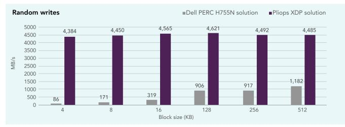
Figure 2: Random write bandwidth, in MB/s, at multiple block sizes for the Pliops XDP and Dell PERC H755N front NVMe solutions. Higher numbers are better. Source: Principled Technologies.
