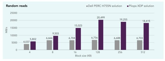
Figure 1: Random read bandwidth, in MB/s, at multiple block sizes for the Pliops XDP and Dell PERC H755N front NVMe solutions. Higher numbers are better. Source: Principled Technologies.
