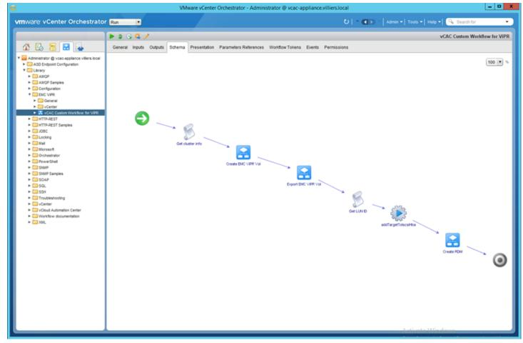
Figure 22: Behind the scenes, vCloud Orchestrator (now known as vRealize Orchestrator) uses ViPR Controller to provision and mount RDM storage to newly provisioned VMs.
