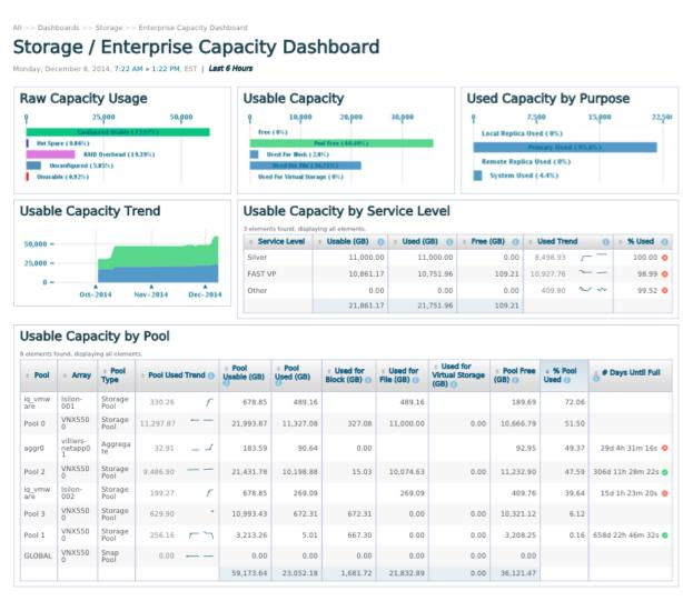
Figure 31: An example Enterprise Capacity Dashboard report in ViPR SRM.
