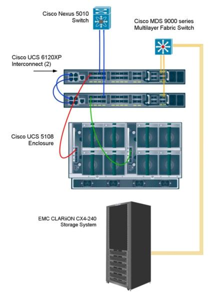
Figure 6: Our test bed configuration for the Cisco Blade Server.
